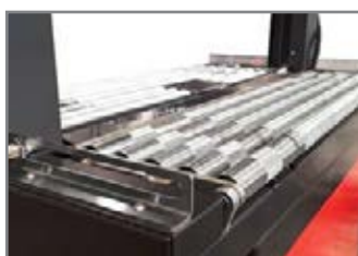
PIANO A RULLI MOTORIZZATI MOTORIZED ROLLER CONVEYOR
