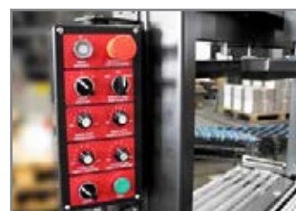
PANNELLO COMANDI ANALOGICO ANALOG CONTROL PANEL
